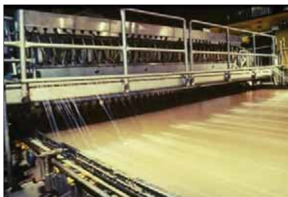
Figure 2 A paper machine headbox in a modern paper making mill
