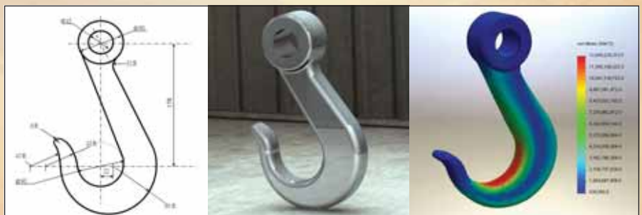
Analyzing the load on a hook using CAD and FEA from 2D to 3D with stress values – useful in validating results obtained by manual calculations.
