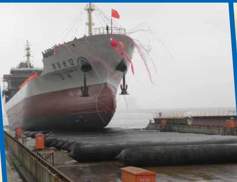
land, etc. Air bags need no extra maintenance and after use they can be cleaned and folded in the corner to wait for another mission. It is easy to find that air bags' elasticity can give more protection to the launched ship. A remarkable character of air bags is that the working height can be changed to redirect the ship or object being launched by adjusting the inner air pressure. For this character it is peerless compared to traditional ship launching techniques.
