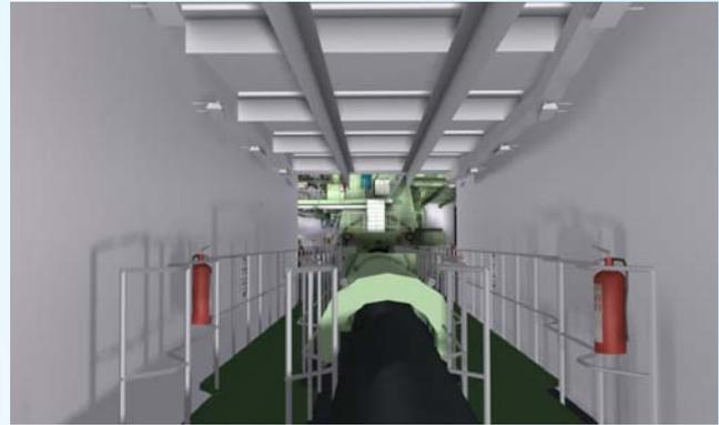
Entire shaft tunnel with moving propulsion engine shaft
