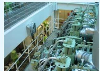
**Real engine made into ER simulator**
