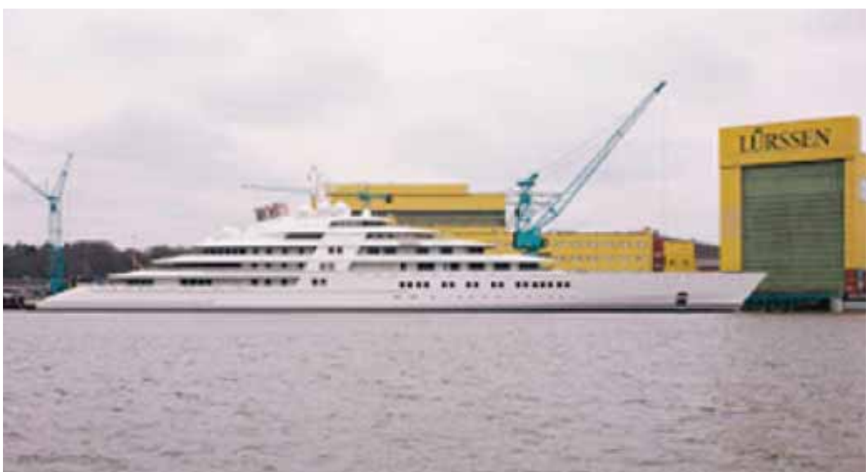
Azzam World's largest launched 180m (590ft) in length and can reach speeds greater than 30kts by a combination of 2 gas turbines and 2 diesel engines with a total of 94000hp
