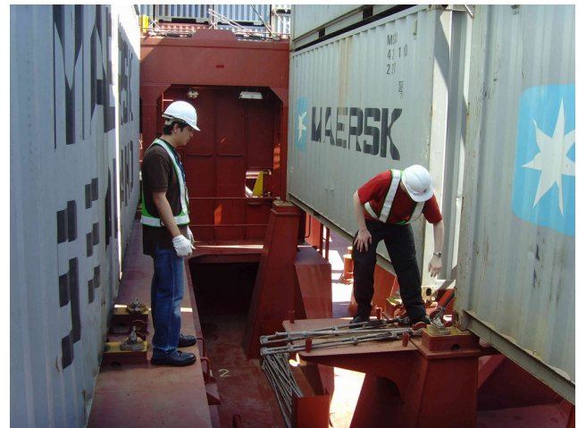
Figure 5: Lashing and unlashings on container ships often requires working in constricted difficult to access spaces with fall hazard. Source: Steamship Mutual.
